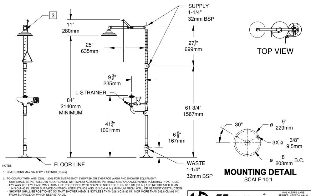
3. DO NOT USE REGULAR PIPE SEALANT. IF NECESSARY USE DOW CORNING 832 SEALANT PLACING 5 SMALL BEADS ON THE MALE THREADS, JUST ABOVE THE FIRST THREAD.
